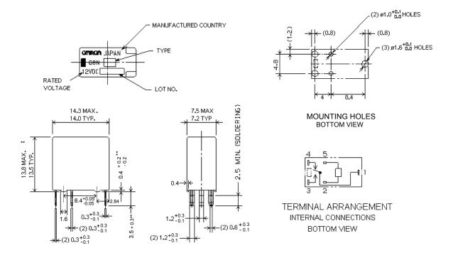
\*\*Note: G8N-17□R types have 0.7mm (not 0.4mm) standoffs for pin in paste process, to make the effective terminal length 3.2+0.3mm (not 3.5+0.3mm), and the height from the bottom of the standoffs to the top of the case 14.1mm MAX, 13.8mm TYP.
