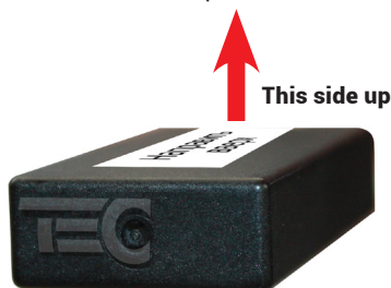
Figure 6. GPS/GLONASS-270 module installation (hermetic)
