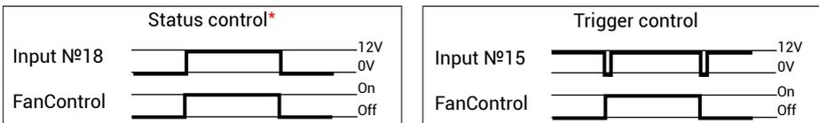
\*To re-enable the system via input № 18- the «status signal» on the input has to disappear and then appear again.
